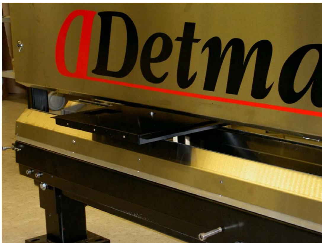
Box for rotating verification disc including pinhole and hole samples.
